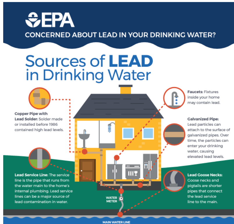
Figure 8-7. Sources of Lead in Drinking Water
